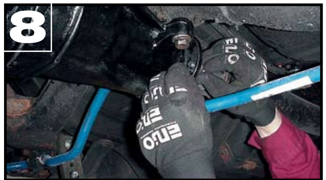
6. The housing cleaned up and bolted back together. 8. Everything is back in place, and bolting in the driveshaft is the last step. PAS
