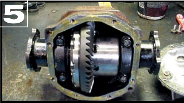
5. Pinion, ring gear and LSD carrier in place. 7. Some Loctite for the driveshaft bolts.
