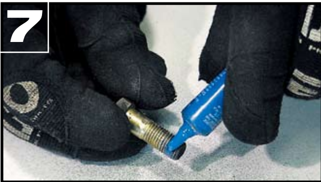
5. Pinion, ring gear and LSD carrier in place. 7. Some Loctite for the driveshaft bolts.
