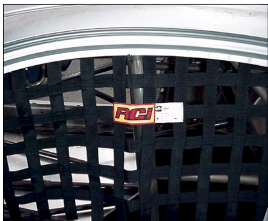
RCI's window net keeps your noggin' in the relative safety of the roll-cage reinforced cockpit.
